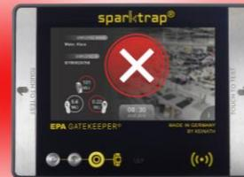
red signaling with „failed“ measurement
